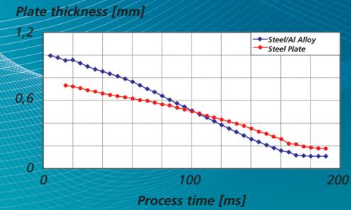
Left: Offline determination of base thickness of joint Al plates; right: Decrease of base thickness of die-sided plate during clinching process
