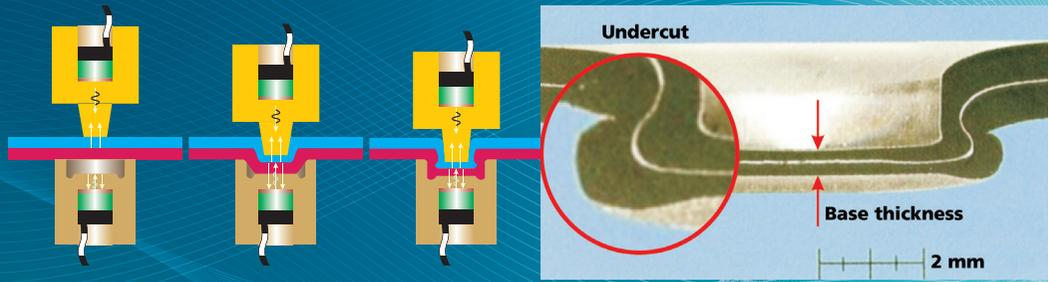
Left: Online determination of the base thickness in clinched joints by ultrasonic methods;
