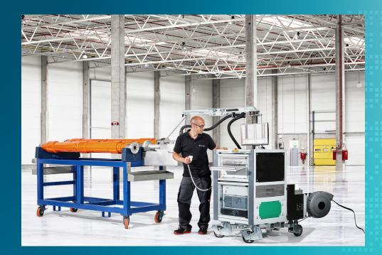
Inspection of wheel set axles with longitudinal bore
