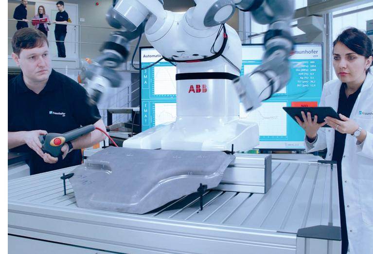
Testing CFRP components using sampling phased array
