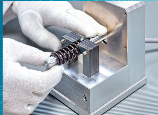
Inspection of valve springs by fully automatic (left) and manual (right) valve spring scanner
