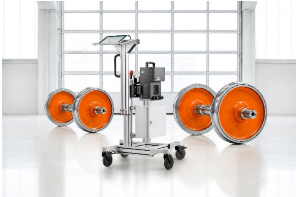
Fig. 1: UER system – Ultrasonic residual stress testing on railway wheels © Fraunhofer IZFP/André Köhl
