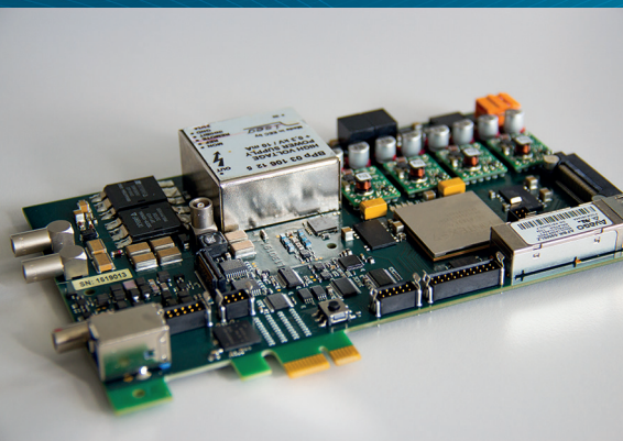
UNIUS board and application LUPUS (air-coupled ultrasound pulser)
