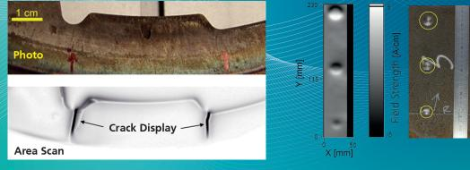
3: Crack visualization after induction hardening; 4: Corrosion inspection
