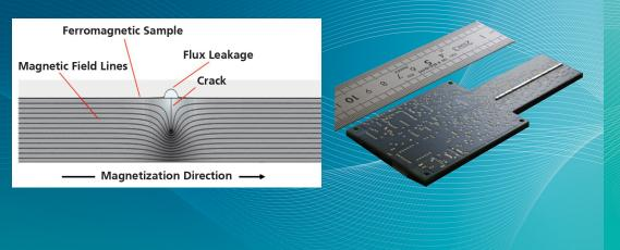
1: Magnetic flux leakage – principle; 2: Linear array of highly sensitive magnetic field sensors
