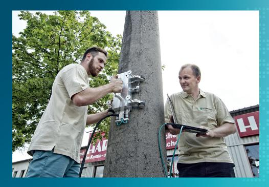
Magnetic flux leakage inspection
