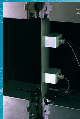
Change of sound velocity of a transmitter / receiver setup as a function of the applied strain of a tensile test; transmitter / receiver setup
