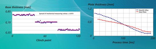
Left: Offline determination of base thickness of joint Al plates; right: Decrease of base thickness of die-sided plate during clinching process
