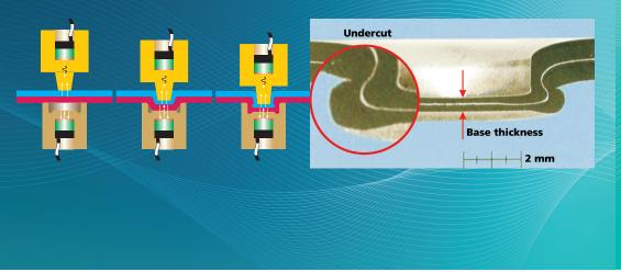
Left: Online determination of the base thickness in clinched joints by ultrasonic methods; right: Undercut and quality feature "base thickness"
