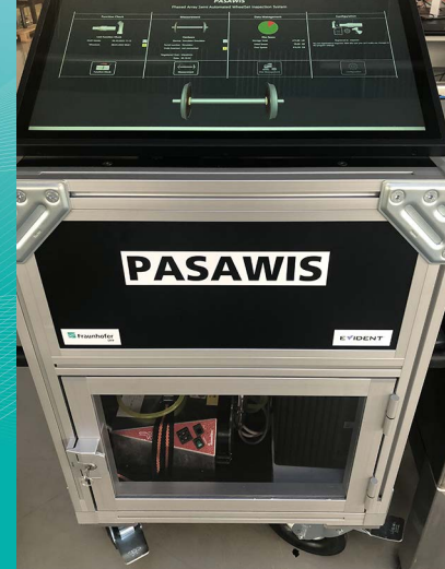
PASAWIS – Mobile manual inspection system for wheelsets
