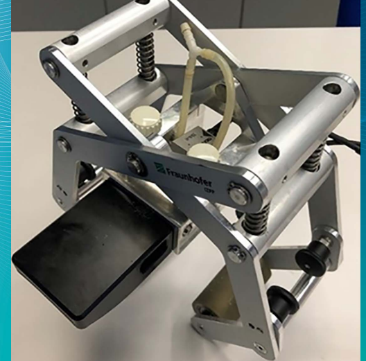
PASAWIS – Mobile manual inspection system for wheelsets
