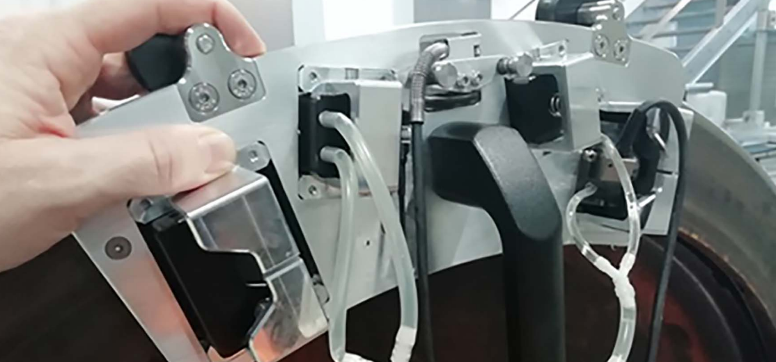
Hand-held scanner for shaft, rim and tread inspection
