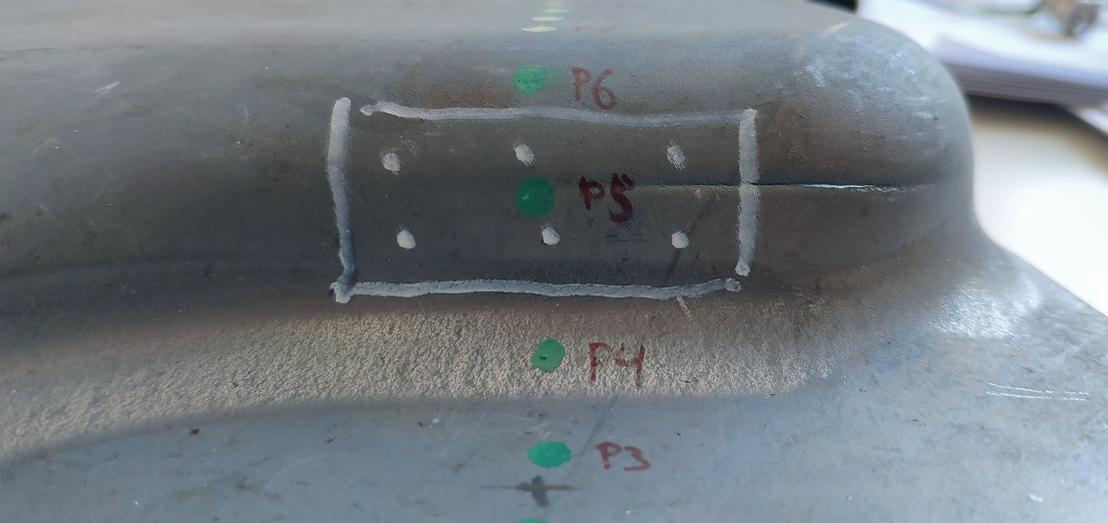
Formed sheet with necking up to the crack
