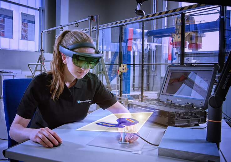
Left: 3D SmartInspect leads the way into the digital NDT world: AR system for manual component testing with automated documentation in DICONDE
