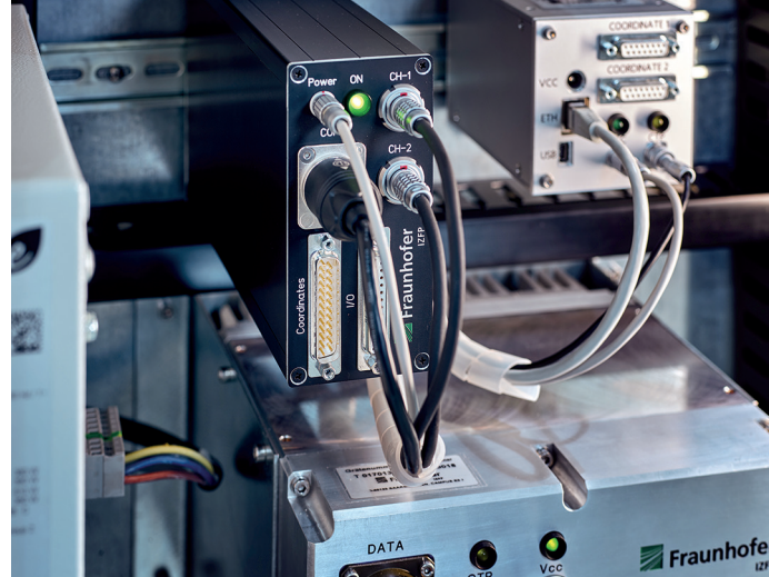
Middle: OPC UA-capable eddy current system (inspECT-PRO); right: eddy current results image
