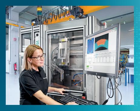
Ultrasound inspection at weld seams of gearbox output shafts
