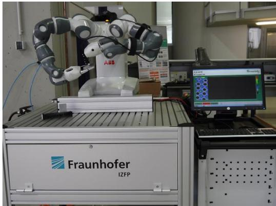
*Robot-assisted sensor system for the nondestructive inspection of hybrid cast components, which can easily be integrated into the quality monitoring of production processes.*
