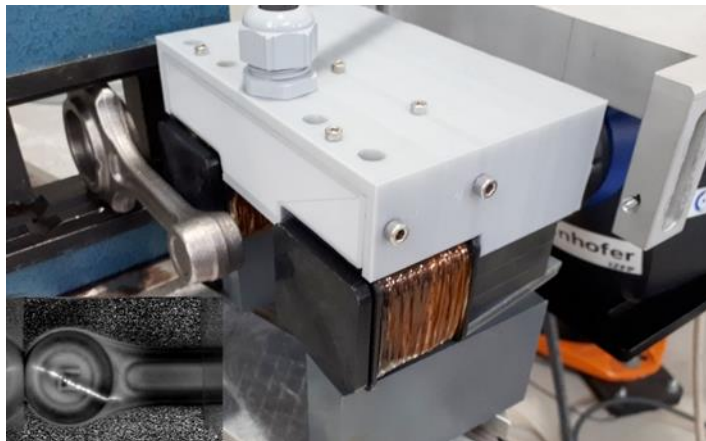
Inspection head for automated detection of surface defects in forged steel parts. Inset bottom left: Thermographic indication of a crack.
