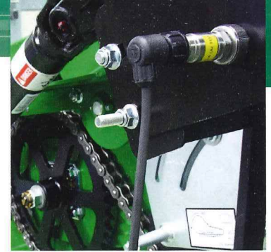
Detailed view of the sound sensor. © Fraunhofer IZFP / Uwe Bellhäuser
