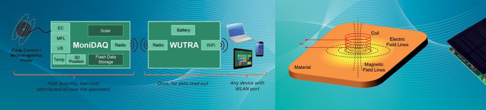
System overview – overview (EC: Eddy Current, MFL: Magnetic Flux Leakage, US: Ultrasound, WiFi – WLAN standard)
