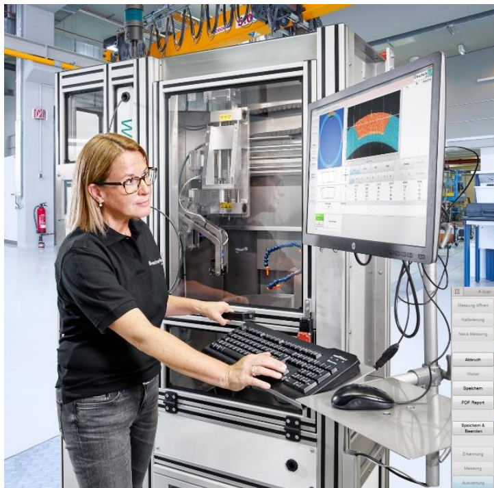
At left: Partially automated system for measuring the weld seam geometry of output shafts for the automatic 8-speed passenger car transmission from ZF Friedrichshafen AG, Saarbrücken factory
