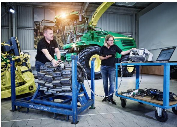
John Deere 8000 Series forage harvester Weld seam testing on blade holder using "LinScanDuo 2.0"
