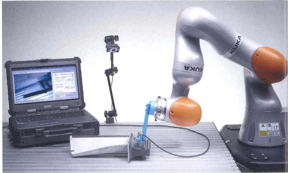
AR system for manual or robot-supported testing of devices or large surfaces.
