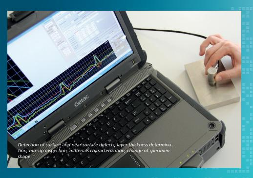
Multi-channel multi-frequency eddy current inspection electronics
