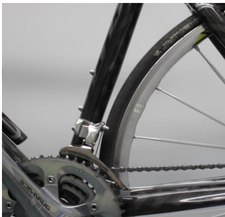
Figure 3: Image of a CFRP frame (“Carbon frame”)
