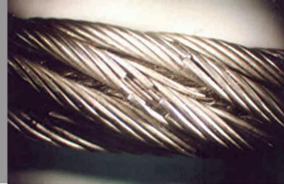
Damaged wire rope (optical image)
