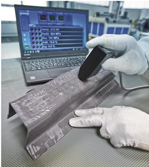
Reliable in-line 3MA inspection results within seconds.
