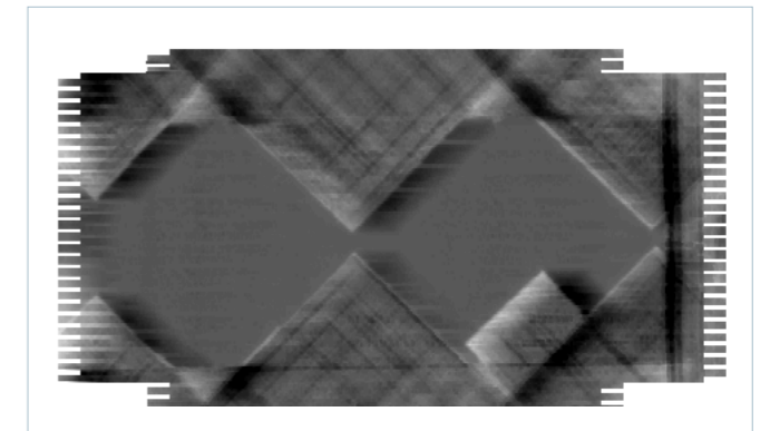
Eddy current testing of a cutted laminate plate right before hybrid Injection-moulding
