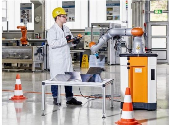
*Realizing robot-assisted inspection of steel sheets for mechanical properties (residual stresses, etc.) by micromagnetic procedures (3MA).*
