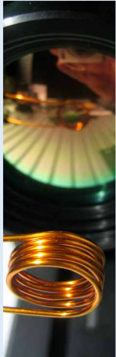
Induction coil in front of an infrared camera
