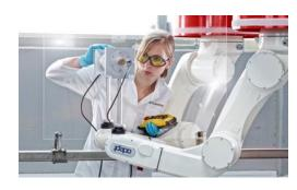
Air-coupled ultrasound: An industrial robot linked to an ultrasound inspection system scans the component. © Uwe Bellhäuser
