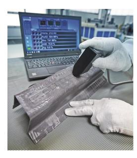
Reliable in-line 3MA inspection results within seconds. © Uwe Bellhäuser
